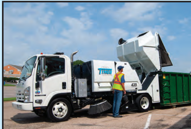
Dumping into a Low-Profile 30-yard Container
