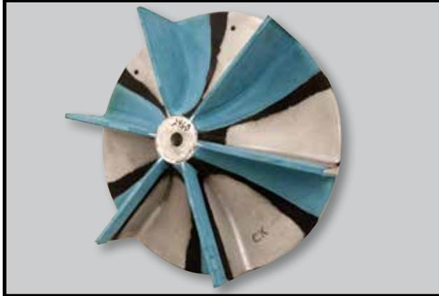
TYMCO blower wheels are cast of high grade (no re-melt) aluminum alloy in a permanent mold. The sand molding method used by most "Copy Cat" companies produces a rough, porous finish with less density than a part produced in a permanent mold. Both the inside and outside diameters of the TYMCO blowers are Computer Numerical Controlled (CNC) machined to produce perfect concentricity and precise tolerances.
