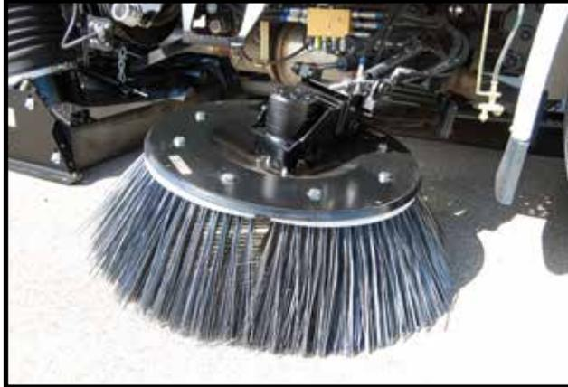
Feedback from the field has proven that the same short life problem holds true concerning gutter broom bristles purchased from “Will-Fit” companies. Our vertical digger filler elements are of high carbon, patented wire. This type of high quality material and construction gives gutter brooms significantly longer life in everyday applications.
