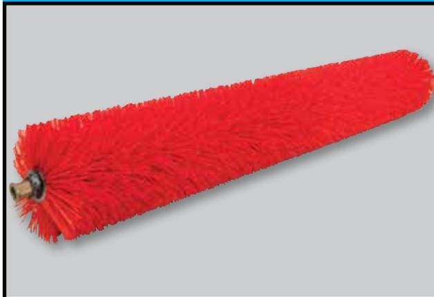
The TYMCO Broom Assist Head (BAH) standard rotary broom is constructed of virgin polypropylene bristles, each having a diameter of .078 and forming a 12 inch diameter around a schedule 40 pipe. Unlike “will-fit” brooms, every TYMCO BAH broom comes with a new bronze hub helping deliver excellent performance every time. Will-fit” brooms either do not come with a new hub or may come with a weaker plastic hub.
