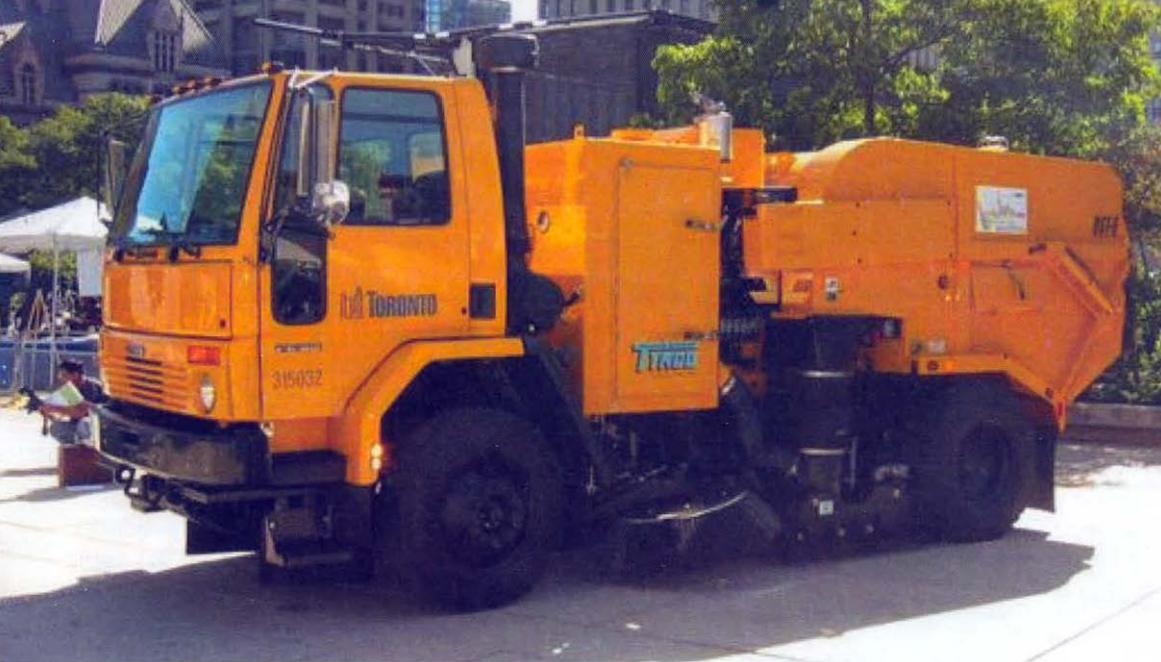
**Toronto cleans up its streets and skies with a new approach to sweeping that keeps particles from being thrown into the air**
