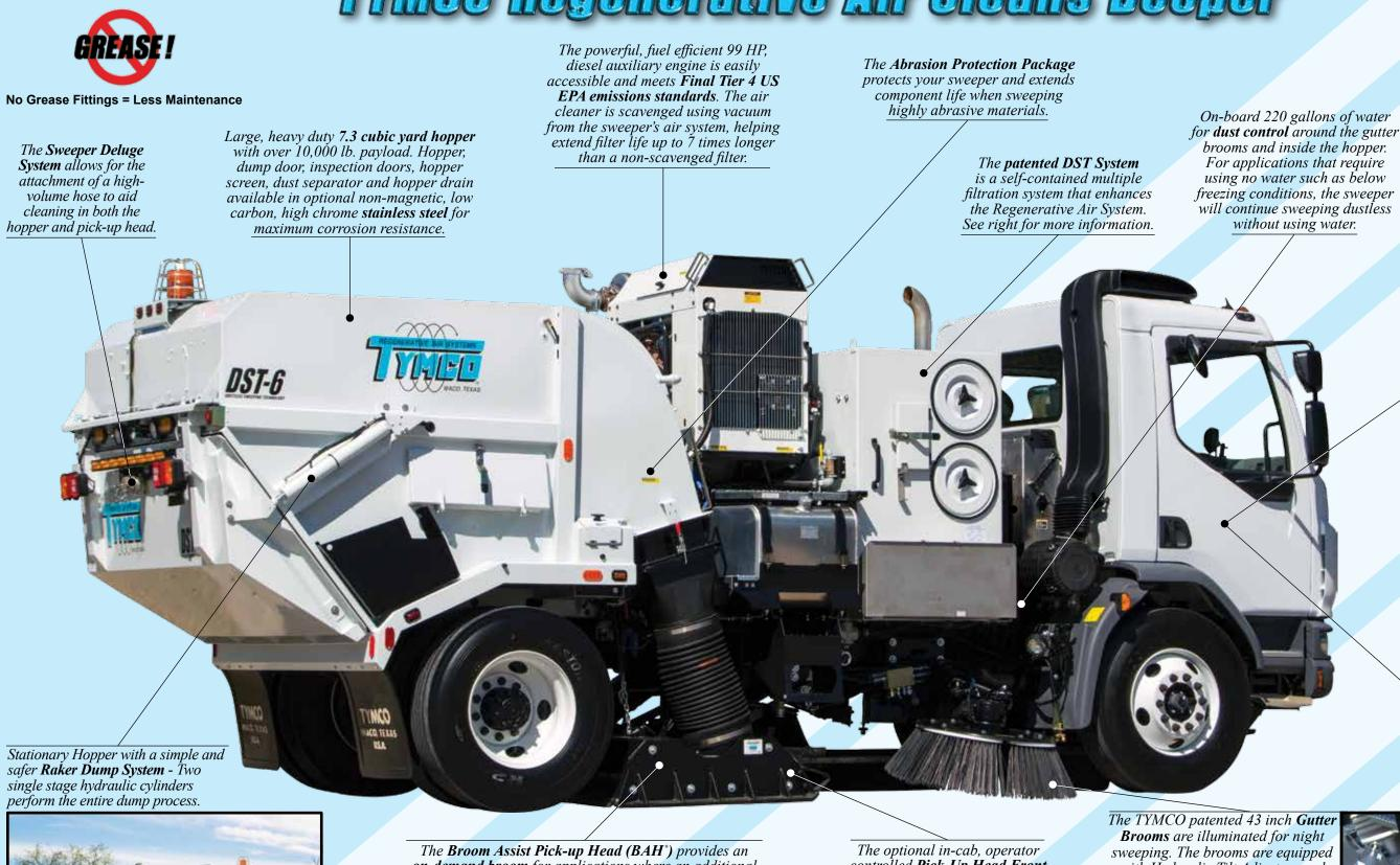
on-demand broom for applications where an additional broom may be desired. In-cab controls allow for broom assisted sweeping only when needed, reducing broom wear.
