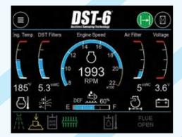
The high resolution color touchscreen display delivers on-board diagnostics for the TYMCO BlueLogic<sup>®</sup> Control System and the auxiliary engine's ECU (Engine Control Unit). Service reminders are displayed for the auxiliary engine and hydraulic system *fluids and filters.*
