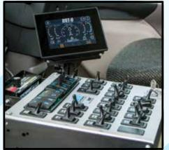
In-cab controls are center mounted and illuminated for ease of operation from either driving position. Switches integrate multi-color LEDs giving operators instant feedback on sweeper functions.
