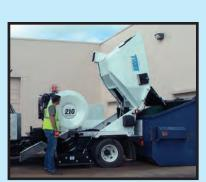
door lets you dispose of bulky items quickly and safely into most 6 and 8 yard dumpsters or containers. The Hopper Drip Edge Extension extends reach for cleaner dumping.
