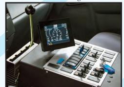
**In-cab controls** are center mounted and illuminated for ease of operation from either driving position. Switches integrate multicolor LEDs giving operators instant feedback on sweeper functions.
