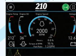
The color touchscreen display delivers on-board diagnostics for the TYMCO BlueLogic® Control System and the auxiliary engine's ECU (Engine Control Unit). Service reminders are displayed for the auxiliary engine and hydraulic system fluids and filters.
