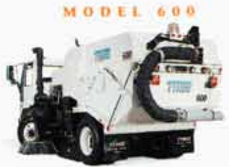
Model 350/600 – Designed for general sweeping applications found on and off the runway. 600 BAH – Offers the same features as the Model 600, but with an on-demand broom assisted pick-up head, especially effective in construction situations and extreme curb and gutter applications.
