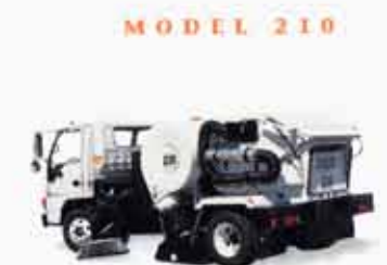
Model 210/300 – More compact, highly maneuverable sweepers designed specifically for use around parking and maintenance areas, airport roads, hangars, and low clearance terminal areas (such as passenger air bridges).
