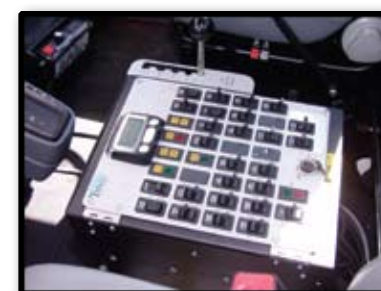
In cab controls are center mounted and illuminated for ease of operation from either driving position.
